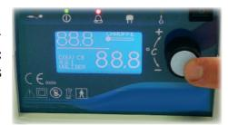
Set by turning the button in the direction "+" and "-" the temperature chosen by the doctor between 30 and 40°C.
