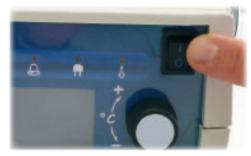
The control unit's electronics then automatically switch to safety mode: all lights are on and the audible alarm sounds.
